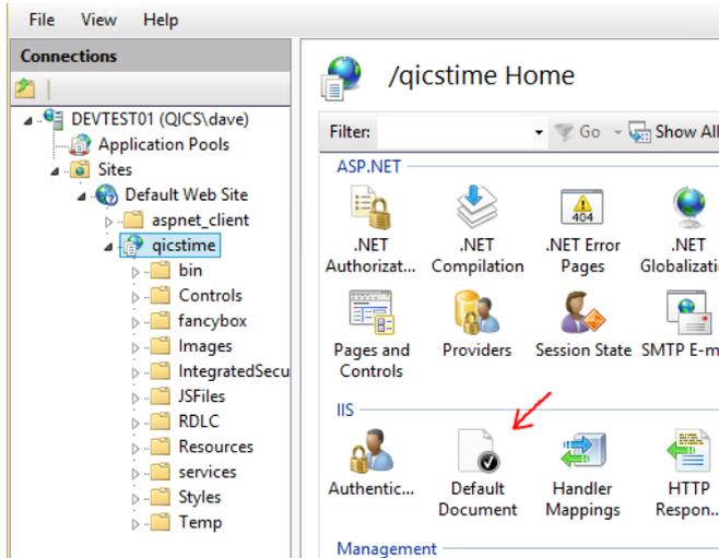
On the QicsTime Web application the “Authentication” section should be configured as shown.
