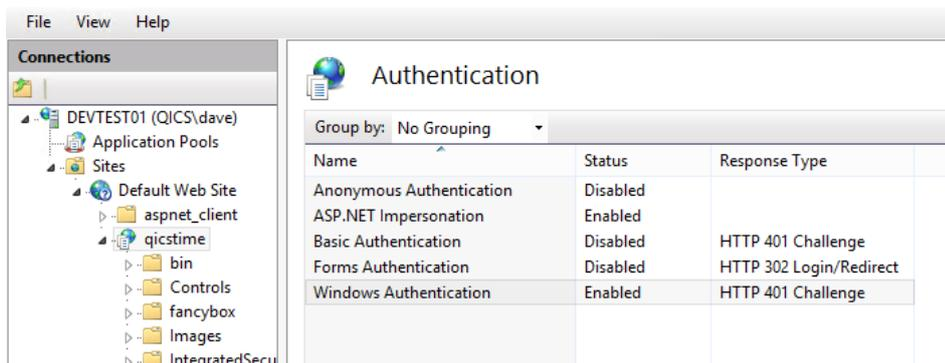
Also make sure that the folder “..\QicsTime\services” accepts anonymous access. The web services and the Mobile application make use of its own authentication and authorization. To check if the QicsTime services are working correctly open the URL:
