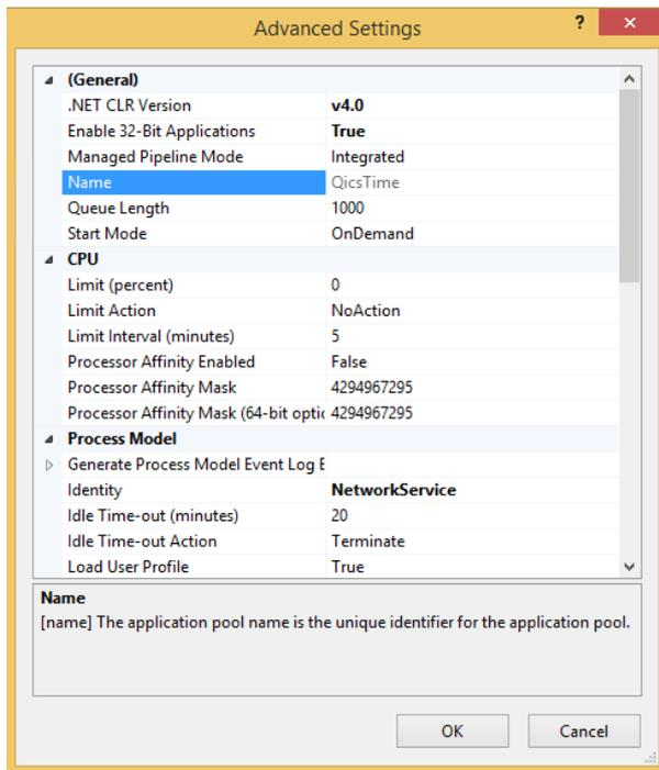
Note that for QicsTime Web it is necessary to set “Enable 32-Bit Applications” to “True”
