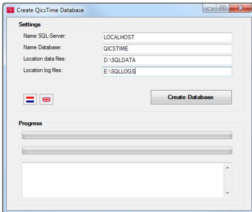
Enter the name of the SQL server, the name of the database and click “Create Database” to start the creation procedure. Change the location of the database and log files if you want, but make sure the folders are correct.
